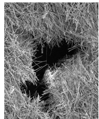
Filter media damage from Electrostatic Discharge (ESD).
